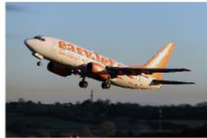
Fig.C.11: Boeing 737-700: 30 kWh per 100 p-km. Foto © Tom Collins
