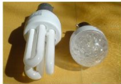
Fig.9.4: Philips 11W naast Omicron 1,3W LED
